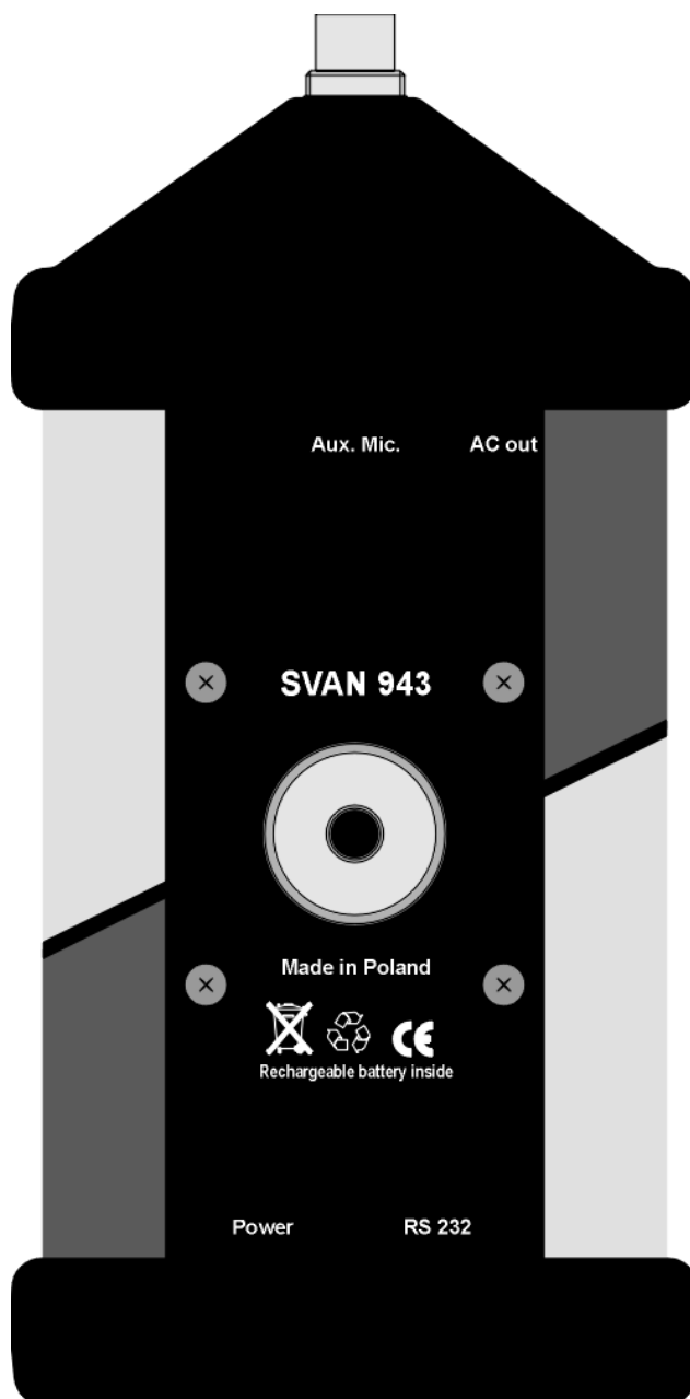
The view of the rear panel of SVAN 943 instrument in 1:1 scale
