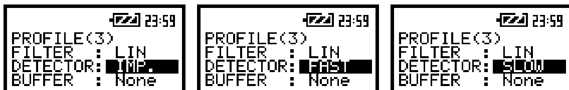
The view of the displays in the PROFILE 3 sub-window; the selection of the detector time constant
