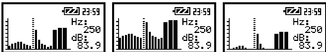
The view of the displays in 1/1 OCTAVE analysis with the shifted horizontal axis in relation to vertical one
