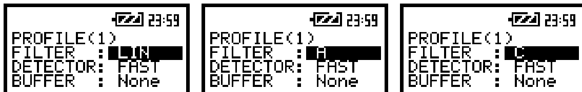
The view of the displays in the PROFILE 1 sub-window; the selection of the weighting filter
