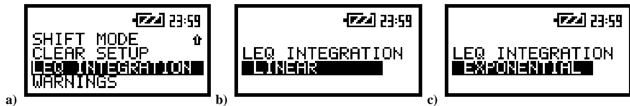
The displays in the SETUP window (a) and with the possible options of LEQ INTEGRATION sub-window (b), (c)
