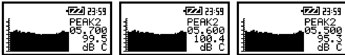
The displays in the PLOT presentation mode; the overview of the values earlier stored in the buffer
