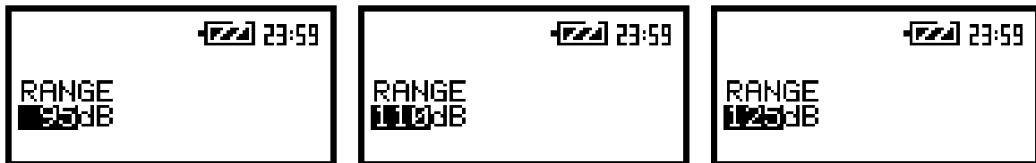
The view of the displays with the RANGE window in 1/3 OCTAVE analyser
