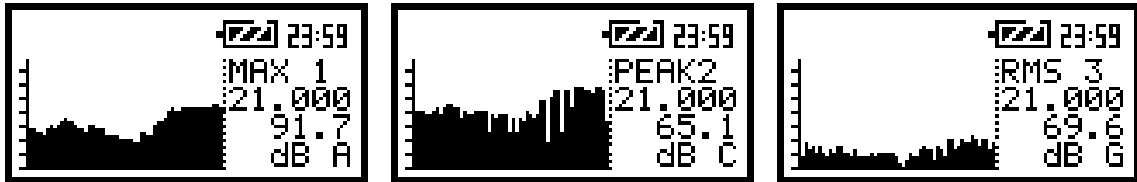
The view of the displays in 1/1 OCTAVE analysis in the PLOT mode; the registered results from all profiles
