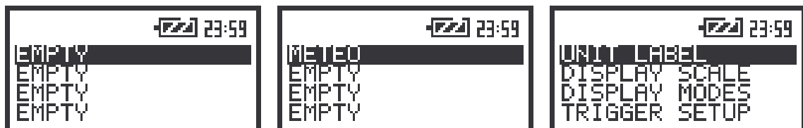
The view of the screens with the sub-lists which were lately accessed by the user (after double pressing of the <MENU> push-button)
