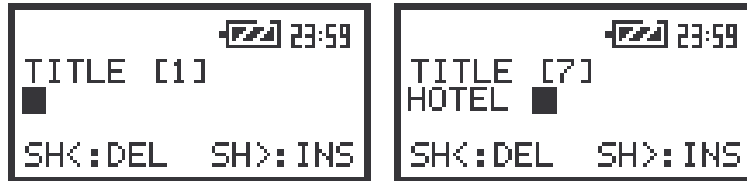
The screens during the edition of the text which has to be printed as a header in the measurement reports
