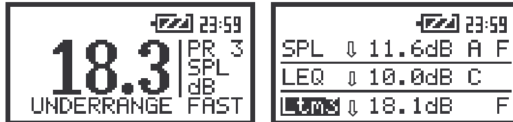
The view of the screen when the level of the measured signal is too low
