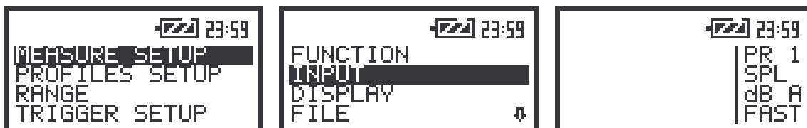
The screens after three consecutive pressing of the <ESC> push-button from the MEASURE SETUP sub-list
