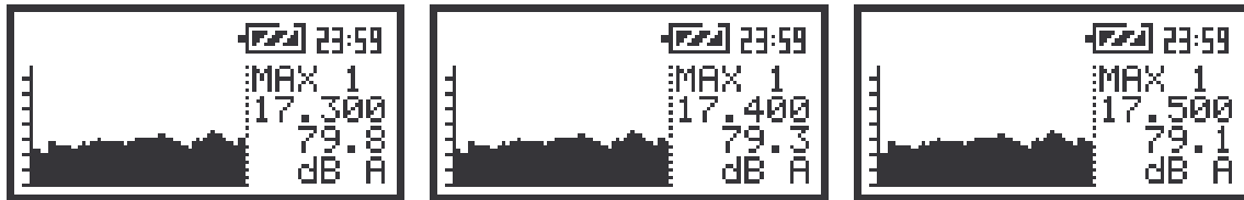
The screens in the PLOT presentation mode; the overview of the values later stored in the buffer
