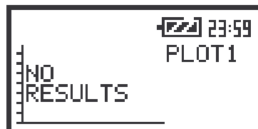
The view of the screen in the PLOT mode when there is nothing in the buffer to be displayed (after setting PLOT as active)
