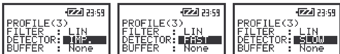
The view of the screens in the PROFILE 3 sub-list; the selection of the detector time constant
