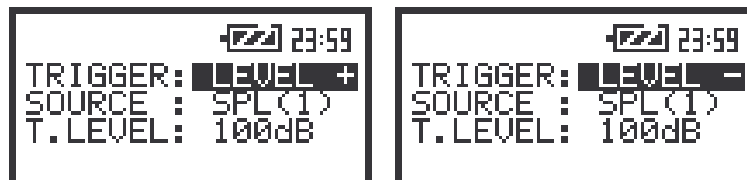
The view of the screens in the TRIGGER SETUP sub-list with the LEVEL modes selected
