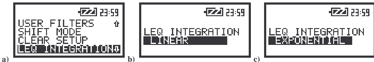
The view of the screens in the SETUP list (a) and with the possible options of LEQ INTEGRATION position (b), (c)
