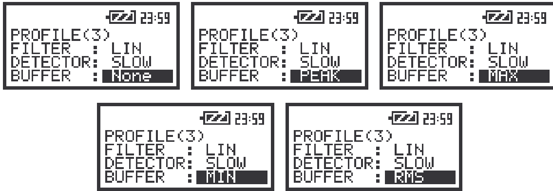
The view of the screens in the PROFILE 3 sub-list; the selection of the result to be saved in the buffer
