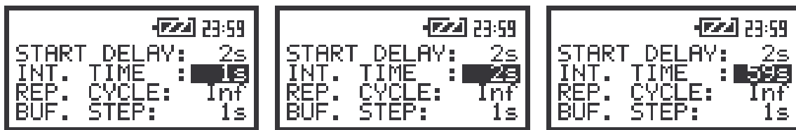
The view of the screens during setting the INT. TIME position; time expressed in seconds
