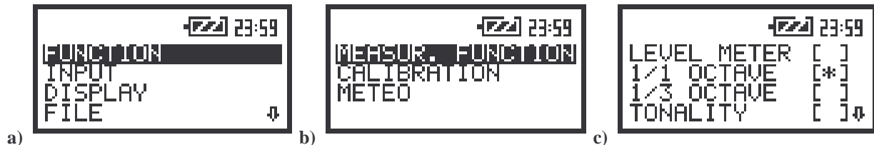
The view of the screens in the main list with the FUNCTION text selected (a), the FUNCTION list opened with the MEASUR. FUNCTION text selected (b), 1/1 OCTAVE analysis mode selected in MEASUR. FUNCTION sub-list (c)
