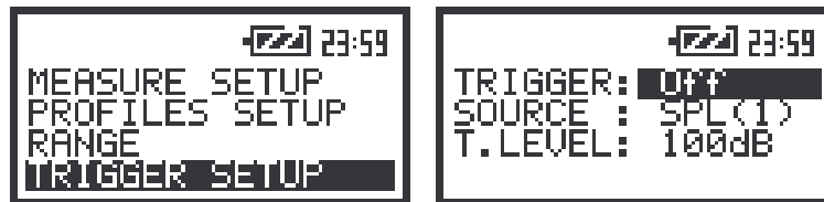
The view of the screens in the TRIGGER SETUP sub-list
