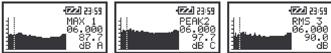
The screens in the PLOT presentation mode; the overview of the values earlier stored in the buffer
