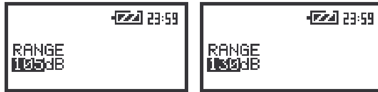
The view of the screens with the RANGE position in 1/1 OCTAVE analyser
