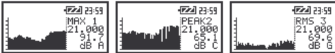
The view of the screens in 1/1 OCTAVE analysis in the PLOT mode; the registered results from all profiles
