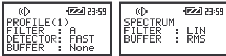
The view of the screens with not accessible parameters of the PROFILES SETUP lists
