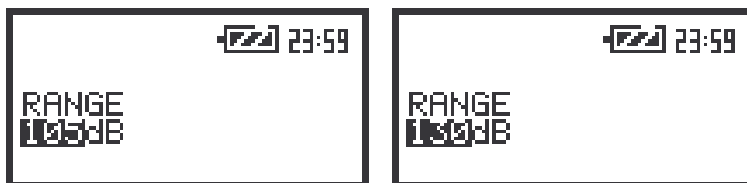
The view of the screens with the RANGE position in 1/3 OCTAVE analysis mode
