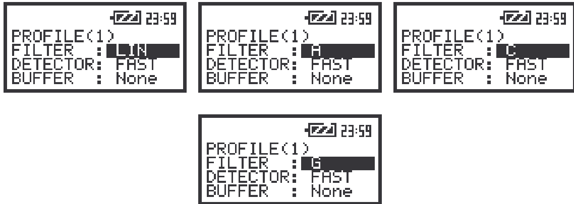
The view of the screens in the PROFILE 1 sub-list; the selection of the weighting filter
