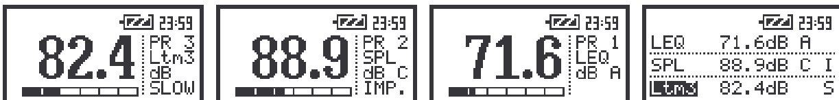
The view of the screens in 1/3 OCTAVE analysis in one profile and 3 PROFILES modes of result's presentation
