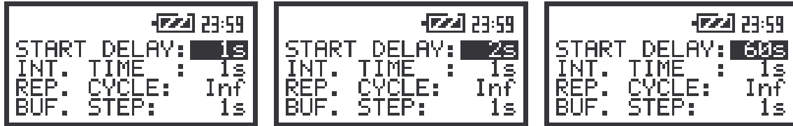
The view of the screens with the MEASURE SETUP sub-list opened; the setting of the START DELAY position
