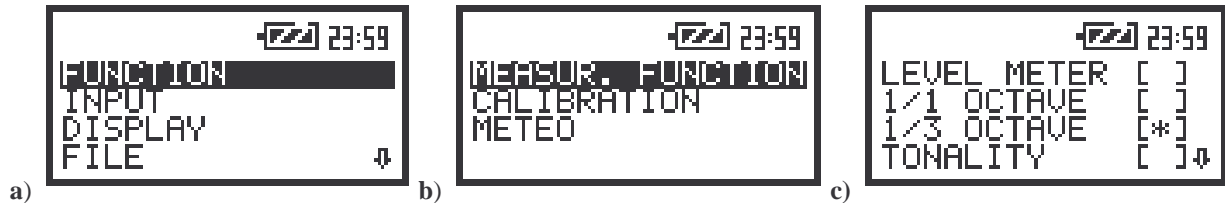
The view of the screens in the main list with the FUNCTION text selected (a), the FUNCTION list opened with the MEASUR. FUNCTION text selected (b), 1/3 OCTAVE analysis mode selected in MEASUR. FUNCTION sub-list (c)
