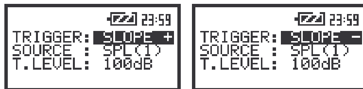
The view of the screens in the TRIGGER SETUP sub-list with the SLOPE modes selected
