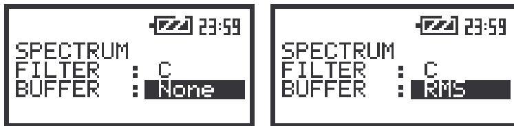
The view of the screens in the SPECTRUM sub-list, the selection of the BUFFER position
