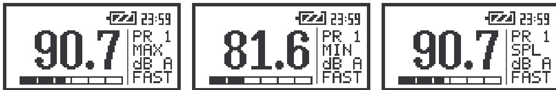
The view of the screens in one profile presentation; the switching between the results in a profile
