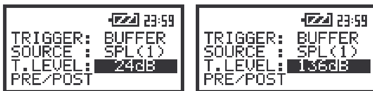
The view of the screens in the TRIGGER SETUP sub-list; the T.LEVEL setting
