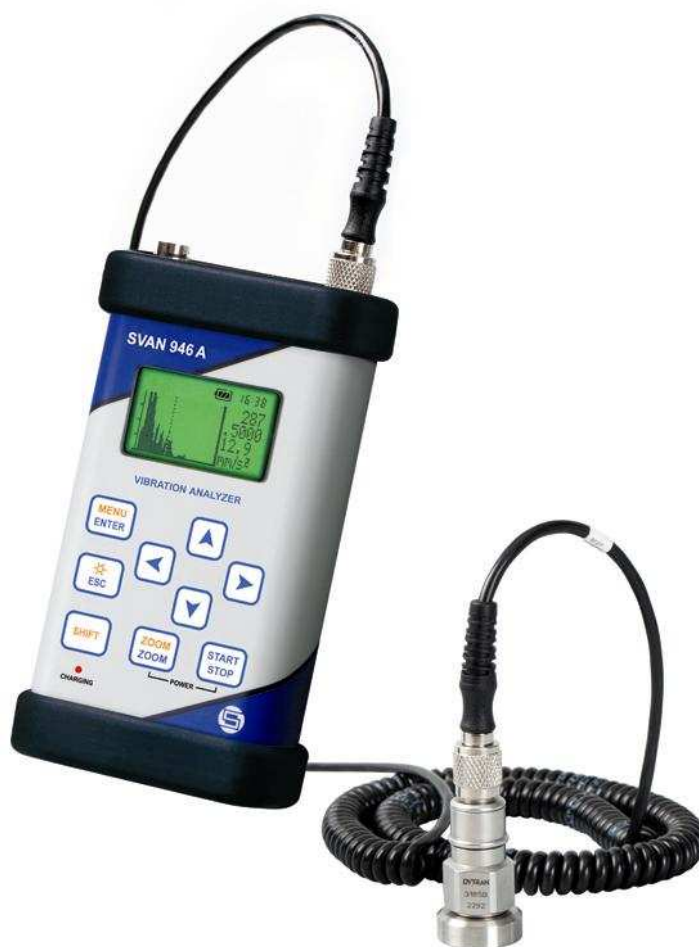
The view of the SVAN 946A instrument with a transducer
