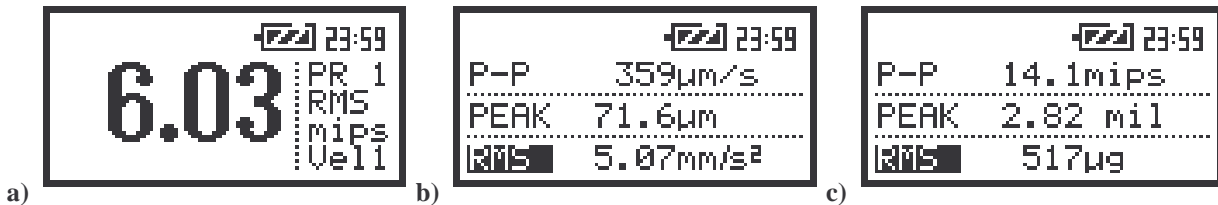
The view of the display in one profile (a) and 3 PROFILES display mode with the vibration measurement results expressed in METRIC (b) and NON-METRIC units (a, c)
