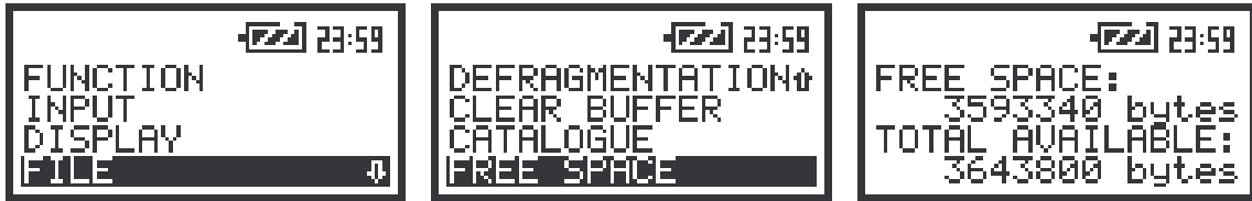
The view of the displays during and after the accessing the FREE SPACE window (path: MENU / FILE )
