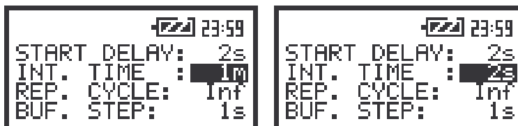
The displays with the INT.TIME position accessed after pressing the <◀> or <▶> push-buttons, respectively
