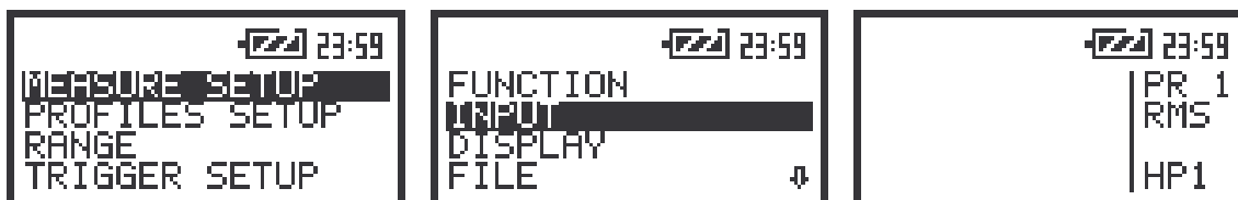
The displays after three consecutive pressing of the <ESC> push-button from the MEASURE SETUP sub-list
