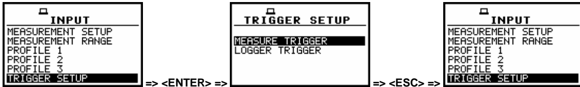
TRIGGER SETUP selected in the INPUT list and the TRIGGER SETUP sub-list
