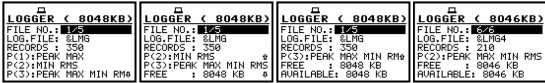
View of the displays with the LOGGER VIEW window; the selection of the file to be seen
