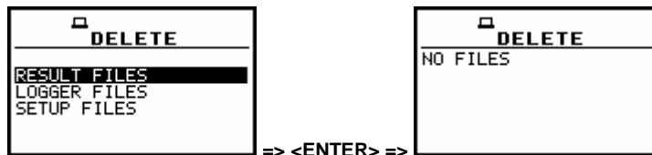
RESULT FILES selected to be deleted and the flash memory does not contain any file
