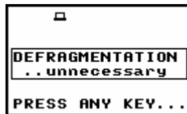
Message in the case when the execution of the DEFRAGMENTATION operation is unnecessary
