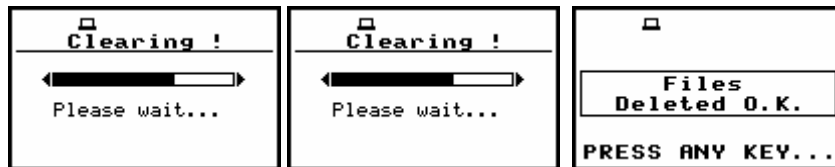
Execution of the DELETE ALL operation for all type files simultaneously
