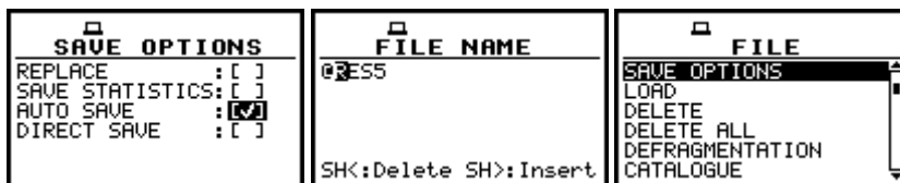
Displays during the execution of the AUTO SAVE switching on; the FILE NAME confirmation and return to the FILE list
