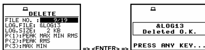
Execution of the &LOG13 file erasing from the logger memory
