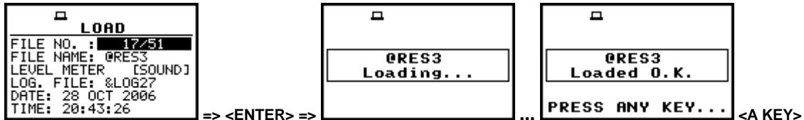
Exemplary displays during a LEVEL METER file loading
