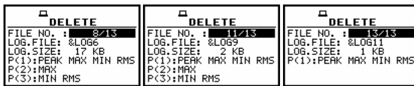
Selection of the LOGGER FILES to be deleted
