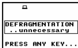
Message in the case when the execution of the DEFAGMENTATION operation is unnecessary
