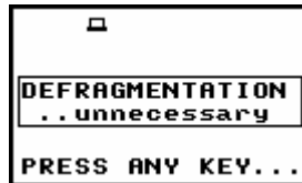
Message in the case when the execution of DEFRAGMENTATION operation is unnecessary
