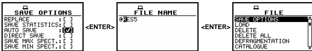
Switching AUTO SAVE on; FILE NAME confirmation and return to FILE window
