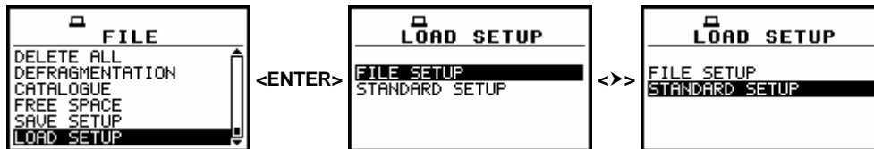
FILE window with LOAD SETUP text highlighted and LOAD SETUP window with available options
