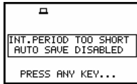
Display after attempt of setting AUTO SAVE option with too short INT. PERIOD
