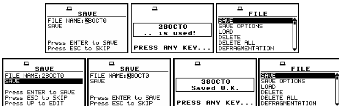
Displays during the attempt of overwriting the existing file, changing the name and saving data
