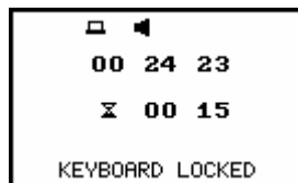
Display after the beginning of measurement when the Key lock is ON
