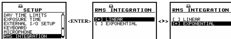
SETUP window with RMS INTEGRATION text highlighted and displays with the available options of RMS INTEGRATION
