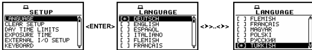
SETUP window with LANGUAGE text highlighted and LANGUAGE windows with all available languages
