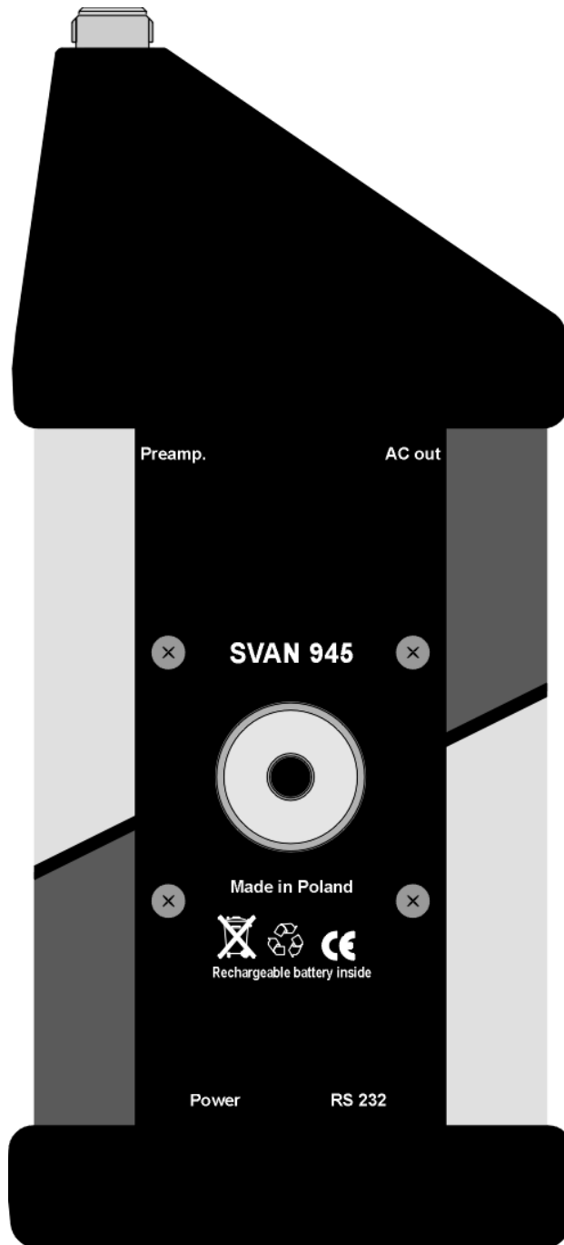
The view of the rear panel of SVAN 945 instrument in 1:1 scale
