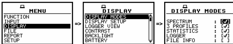
Main list, DISPLAY list and DISPLAY MODES window with available modes of presentation
