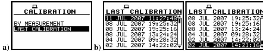
CALIBRATION list with LAST CALIBRATION text selected (a) LAST CALIBRATION window opened with ten calibration records (b)
