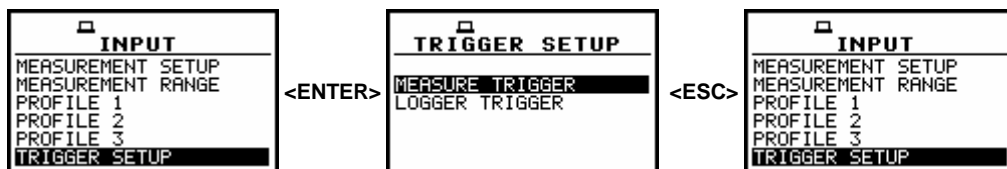
TRIGGER SETUP selected in the INPUT list and the TRIGGER SETUP sub-list
