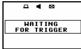
Display when the instrument is waiting for the trigger conditions fulfilment
