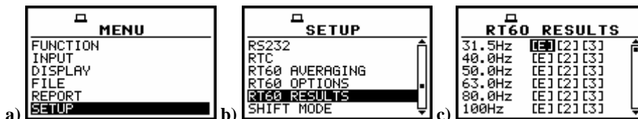
Main list with SETUP text selected (a), SETUP window with RT 60 RESULTS text highlighted (b), RT60 RESULTS window (c)
