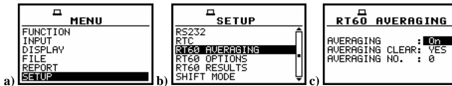
Main list with SETUP text selected (a), SETUP window with RT 60 AVERAGING text highlighted (b), RT 60 AVERAGING window (c)
