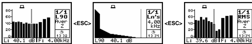
1/1 OCTAVE spectrum of LN, after return to the presentation of the statistical analysis results performed for selected 1/1 OCTAVE filter and after return to the presentation of 1/1 OCTAVE spectrum
