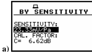
Displays during setting the sensitivity lower than 50.0 mV / Pa with the calculated calibration factor
