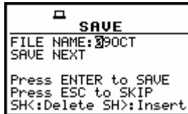
Display during the process of setting the character in the edited name
