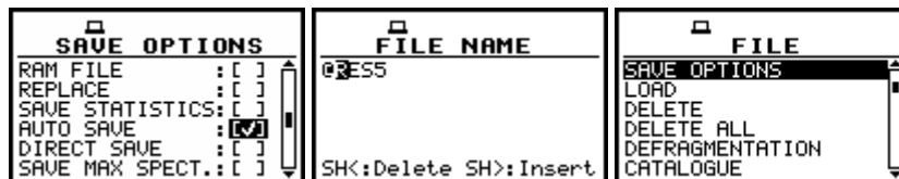
Displays during the execution of AUTO SAVE switching on; FILE NAME confirmation and return to FILE list
