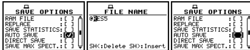
Displays during the execution of AUTO SAVE switching on; FILE NAME skipping and return to SAVE OPTION sub-list
