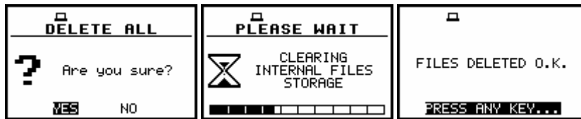
Displays during the execution of DELETED ALL operation and after this execution
