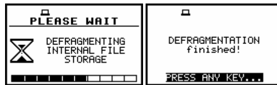
Displays during the execution of DEFRAGMENTATION operation
