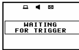
Displays when the instrument is waiting for the trigger conditions fulfilment
