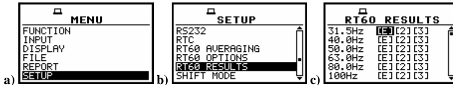
Main list with SETUP text selected (a), SETUP window with RT 60 RESULTS text highlighted (b), RT60 RESULTS window (c)
