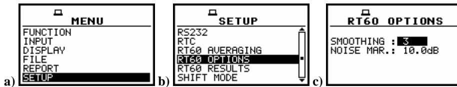
Main list with SETUP text selected (a), SETUP window with RT 60 OPTIONS text highlighted (b), RT 60 OPTIONS window (c)
