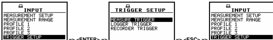
TRIGGER SETUP selected in the INPUT list and the TRIGGER SETUP window
