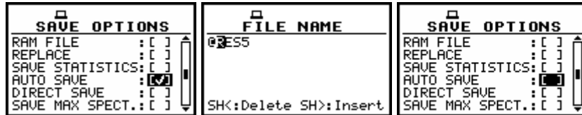
Displays during the execution of the AUTO SAVE switching on; the FILE NAME skipping and return to the SAVE OPTION sub-list
