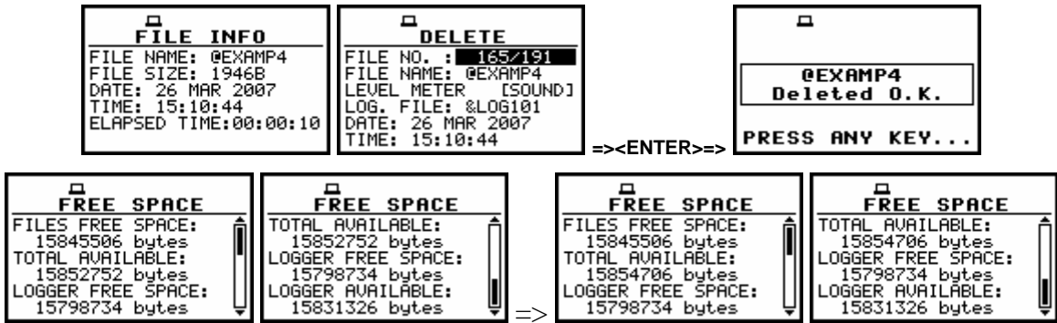
Execution of the @EXAMP4 file deletion and the influence of this process on the memory space
