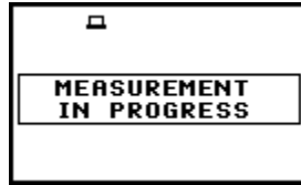
Displays after the attempt to perform an unavailable operation during measurement in progress
