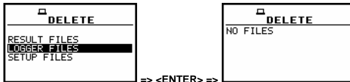
LOGGER FILES selected to be deleted and the memory does not contain any file
